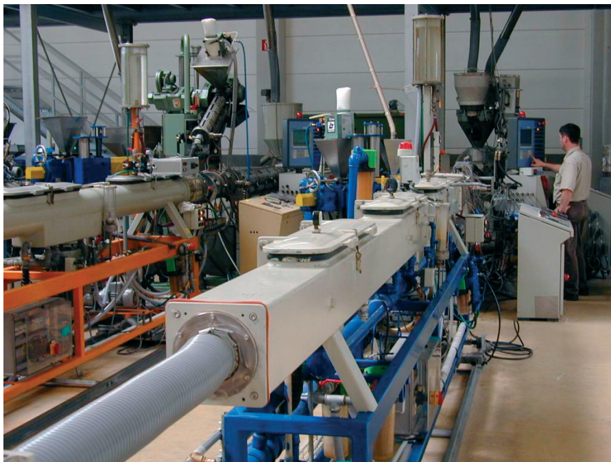
Extruder for pipe manufacture in the Niederwinkling plant
